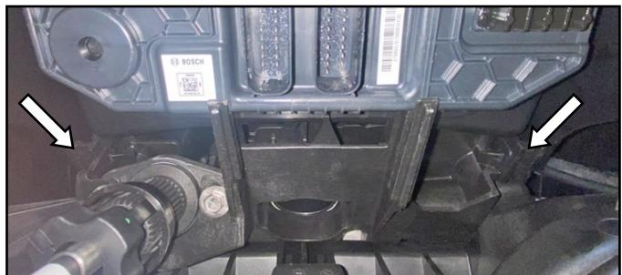
At steering column, remove bolts (2) securing steering column in place. Remove pieces and discard.
