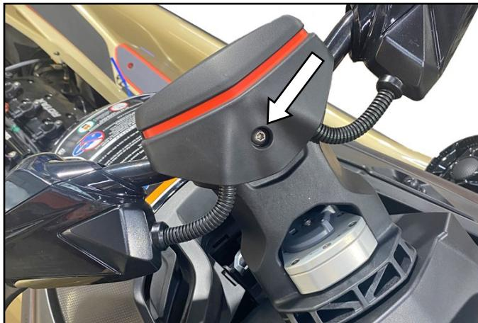
Remove switch (control pad) covers on both sides by prying out and up at designated locations at lower edge on each cover. Set covers aside. **TIP:** Insert small, flat screwdriver behind tab and pry upward.
