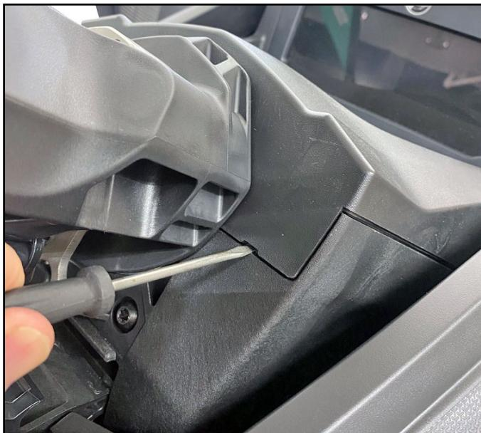
Back inside, at base of digital dash display there are locking tabs securing the display support/steering column cover in place. Pry tabs outward to release display support/steering column cover.
