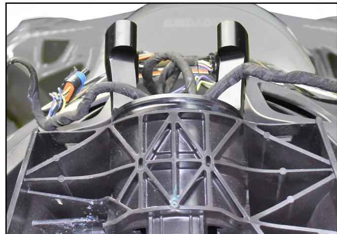
Install aftermarket handlebars and center side to side. Secure handlebars using supplied clamp and M8x25 SHCS (4). **NOTE: Apply red Loctite to threads. Ensure handlebar cross-bar is directly over clamp. Torque bolts evenly in a crisscross pattern to 15 ft•lb (20 N•m).**
