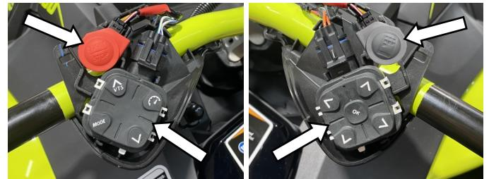
Remove control housings from handlebars (2 Torx screws each side). Save hardware for use later.
